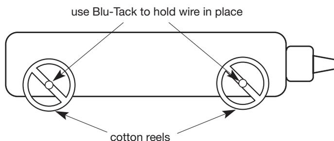
Use an inclined plane or an elastic band between two chair/stool legs to make the dragster move. If you use the elastic band method, the dragster will need to be weighted down – cut a small hole in the washing-up bottle and insert some 100 g masses.
