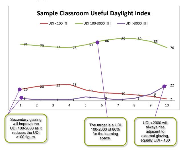
The sample graph here shows the results of a UDI analysis for a classroom. Each line represents the results as if a line had been drawn down the centre of the room from the external window to the back wall. A 3D graph would provide further detail.
